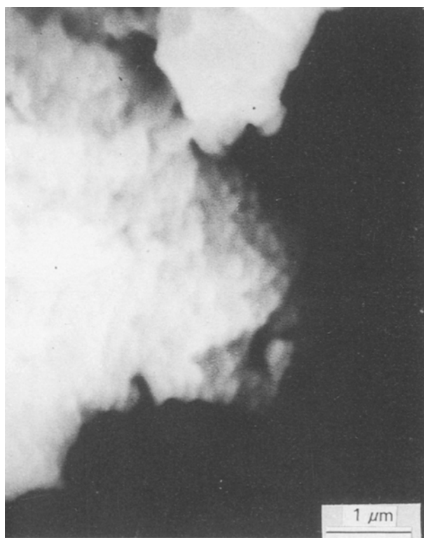
Figure 9 Scanning electron micrograph of PZT particles obtained after the calcination of a mixture of PbCO_3 and (Zr_{0.525}Ti_{0.475})O_2 at 700 °C for 2 h.
